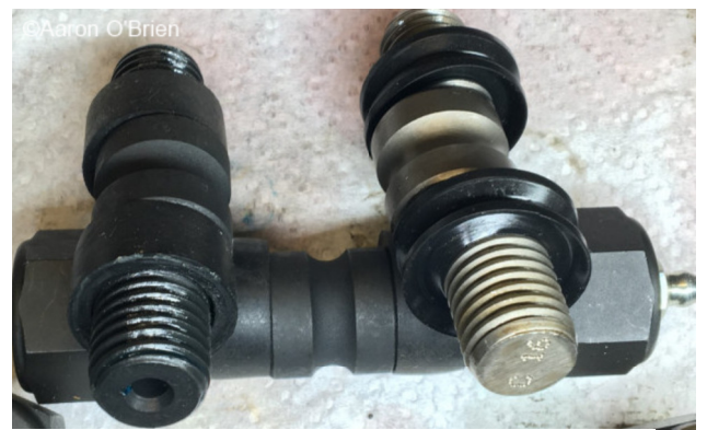
These pictures show two different types of pivot pins. Notice the concentric lobe.
